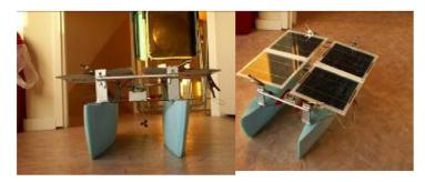
13. First hull design based on DELFTship program
