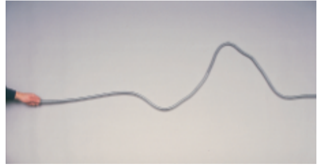
FIGURE 14–4 These two photographs were taken 0.20 s apart. During that time, the crest moved 0.80 m. The velocity of the wave is 4.0 m/s.
