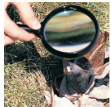
FIGURE 18–13 A converging lens can be used to start a fire in a pile of leaves.
