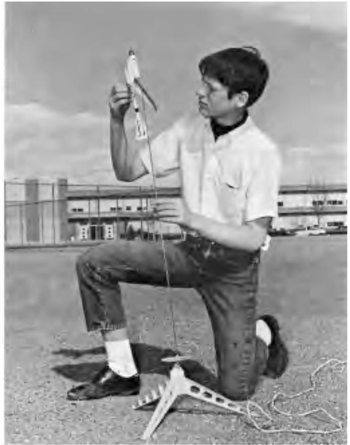
**OR** Continue your boost-glider activities with the construction of a pop-pod boost-glider. This type of glider is propelled by a power pod that separates at apogee and returns on its own parachute. The airframe returns by gliding.
