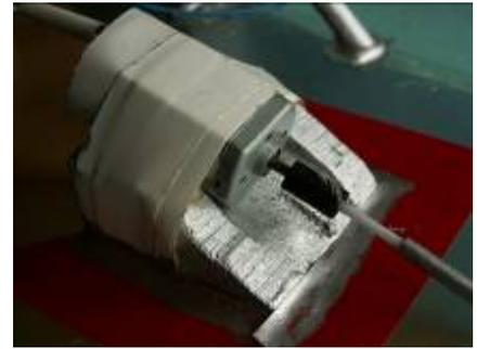
5. Attaching the propeller to the other end of the shaft.
