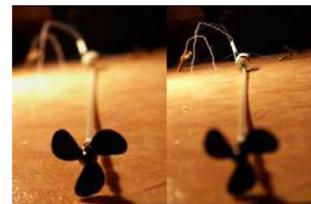
4. Attaching the motor to the deck and connecting it to the shaft which links to the propeller (still to attach)
